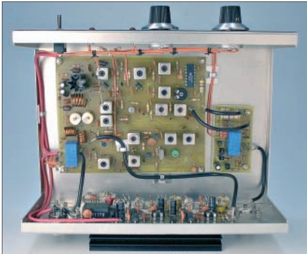
● Fig. 1: An inside view of the TRC4-10iL 28 to 70MHz transceiving converter (transverter). Each well made unit is made-to-order on a two week schedule. The transverter ordered by G3XFD arrived exactly 14 days after he ordered it! (see text).
