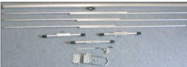
● Fig. 3: The Sandpiper 3-element 70MHz beam antenna arrived in a kit of parts and G3XFD recommends you "don't drop them in long grass"! (see text).
