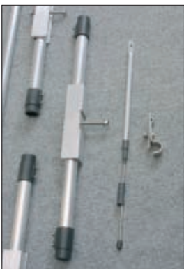
● Fig. 4: Close up view of the main element boom clamps (mid right) and the new 'Trombone' type Gamma match unit and clip (see text).
