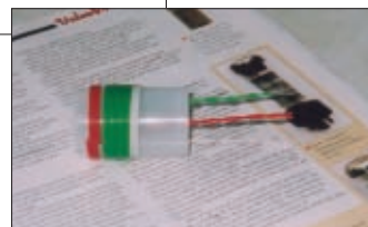
Fig. 3: Photograph showing G4JCP's prototype coil. The grid winding is green (10 turns), the reaction winding red (4 turns) and the antenna coupling winding is white (3 turns).
