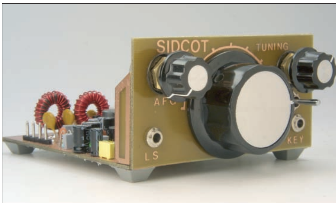
● The completed Sidcot 3.5MHz c.w. transceiver. This month the author and designer Tim Walford G3PCJ describes the transmitter section and the completion of the project. And if you want to make your project a little easier - Tim has prepared a kit which provides a transceiver in the style illustrated.
