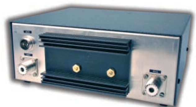
● Fig. 2: Rear panel view of the 70MHz transverter showing power (top left), antenna (lower left) and transceiver (right) connections. The heat-sinking is more than adequate for the single bi-polar transistor power amplifier (p.a.). Each unit comes with an individual calibration for transmit power and receiver gain.
